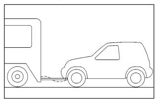
Notice: If you tow a two-wheel-drive vehicle with all four wheels on the ground, the transmission could be damaged. The repairs would not be covered by your warranty. Do not tow a two-wheel-drive vehicle with all four wheels on the ground.
